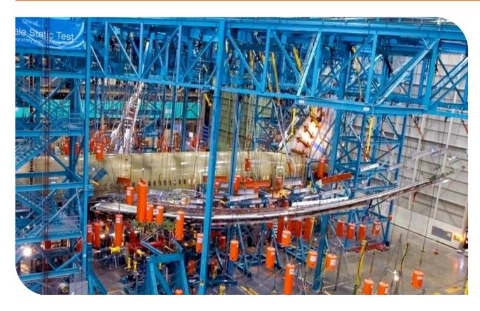
Full scale structural test of Boeing 787
