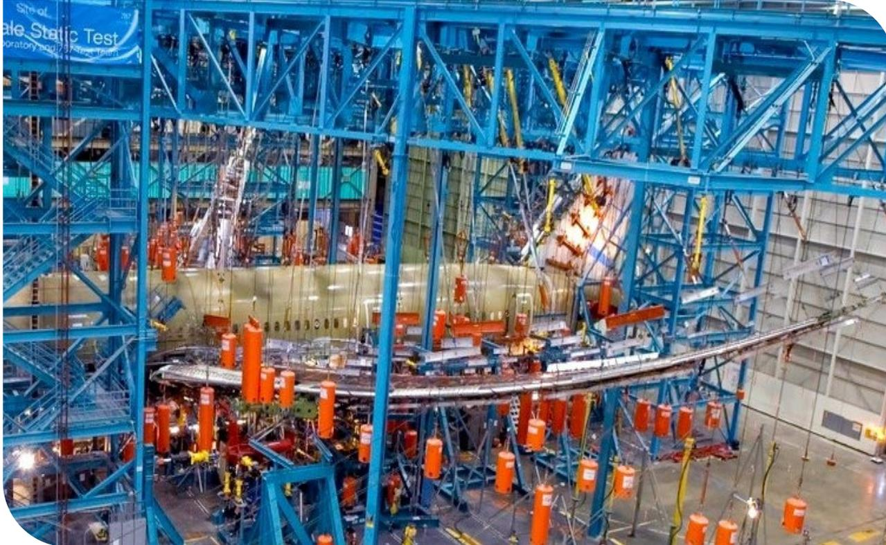
*Full scale structural test of Boeing 787
