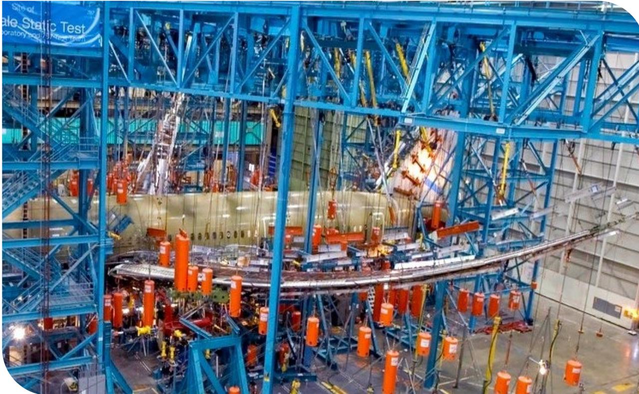
*Full scale structural test of Boeing 787
